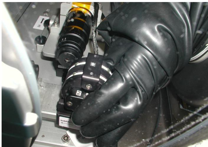
*An InSPACE coil assembly is shown being installed in position for testing. The assembly holds a small vial which contains magnetorheological fluid.*
