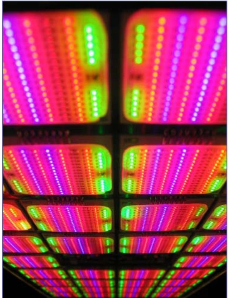
**VEGGIE's LED lighting provides high intensity lighting in a lightweight, thin profile system with tunable frequencies to match biological need.**
